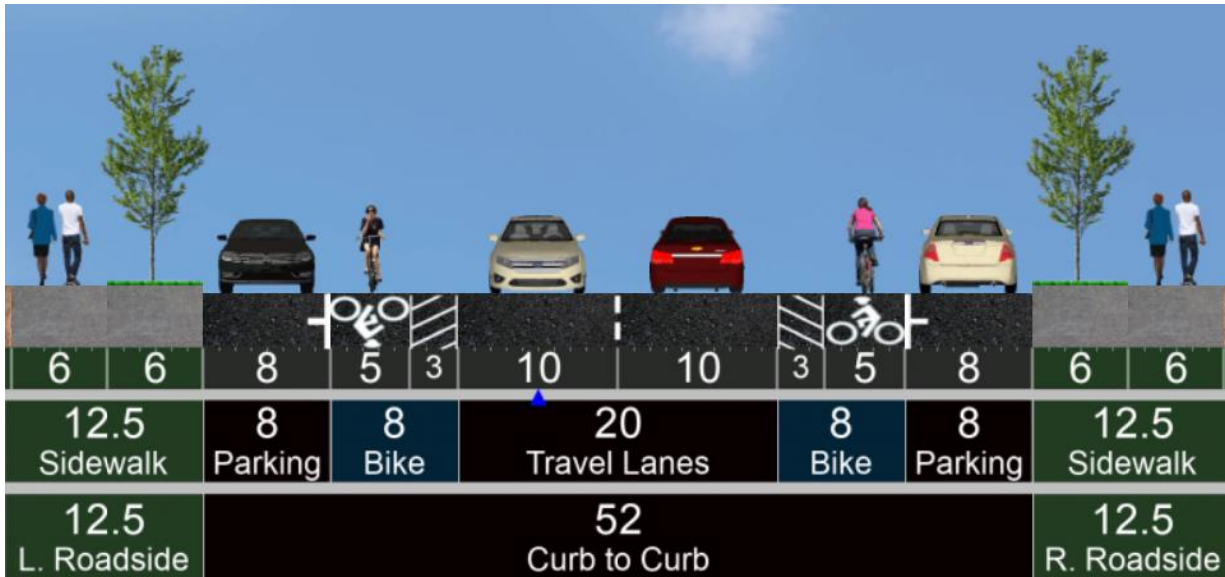
FIGURE 35: TYPICAL CITY COLLECTOR, NEIGHBORHOOD ROUTE, AND LOCAL STREET CROSS-SECTION WITH MAJOR PEDESTRIAN AND NEIGHBORHOOD BICYCLE ROUTE DESIGNATION
